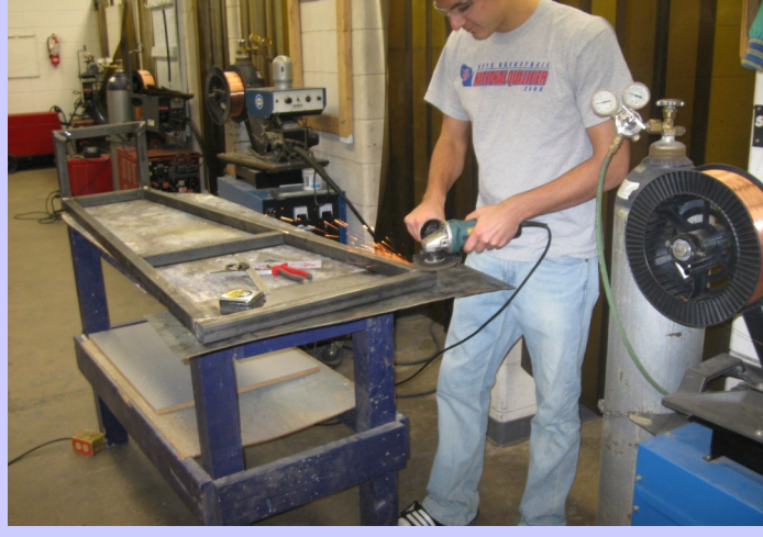
Cole grinding the welds to prepare the surface for attaching the roll bars.
